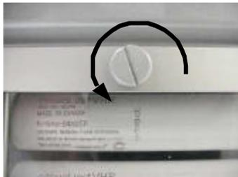
Fig. 3.1 Acrylic panes – Undo screws
