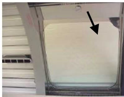
Fig. 3.7 Removing the filter pane frame
