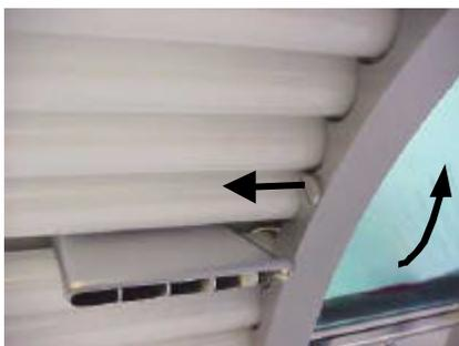
Fig. 3.6 Dismantling the tube covering
