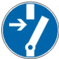
**Before opening the unit switch off the fuses to disconnect the system from the voltage supply!**
