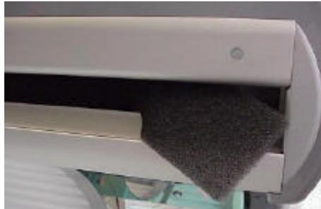
Fig. 3.12 Replacing the filter mat
